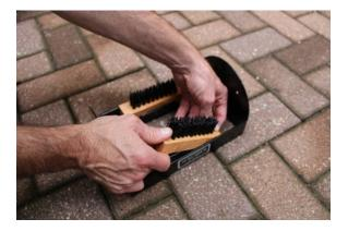
4. Drill new side brushes in with screws (2 screws per side)
