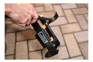
3. Replace bottom brushes with SBM1 Poly brushes inserting into slot wide to narrow end and pounding with hammer to secure (2 brushes)
