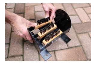
4. Drill new side brushes in with screws (3 screws per side)
