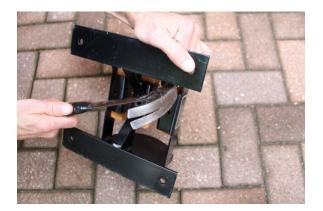
3. Replace bottom brushes with SB5U Nylon brushes inserting into slot wide to narrow end and pounding with hammer to secure (3 brushes)
