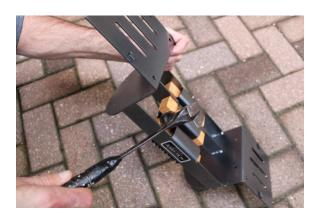
3. Replace bottom brushes with SB5U Nylon brushes inserting into slot wide to narrow end and pounding with hammer to secure (3 brushes)
